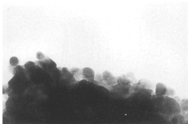
Figure 3 Transmission electron micrograph of \text{HfO}_2 powder heated at 850^\circ\text{C} for 19 h ( \times 300\,000 ).
